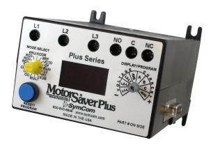
The SymCom 777VA-02 is an electronic overload relay with the same features as a 777-P, with the added convenience of a Restart Delay 1 of 0,2-500 minutes (RD1) and a Under Current Trip Delay of 2-255 minutes (UCTD). These added features are essential for pumps that require a longer restart delay to allow for long back-spin time and for motors with extended soft-start times.
